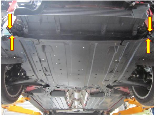
11. With the mounting bracket removed the next step is to undo the two hose clamps securing the rubber hoses to the inter cooler. They have 8mm fastenings which can be loosened off with an 8mm socket and rachet drive or a flat blade screw driver.
