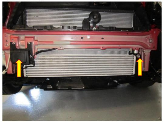
13. Now you will be able to install your new Forge Motorsport intercooler. Carefully angle the intercooler behind the ACC bracket and loosely re fit the two 10mm fasteners to hold the intercooler in place. You can then slide the hoses back on, locate the hoses as you can and the tighten the hose clamps up. Finally tighten the 10 mm fasteners.
