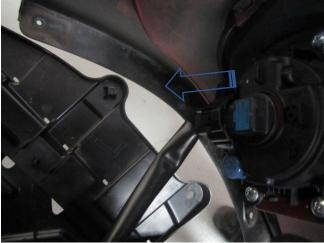
5. Now with the bumper removed you will see the OE intercooler, there is air ducting in front of the intercooler that needs to be removed. First remove the three plastic fasteners running along the top of the air ducting
