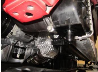
12. The final stage for removal of the OE inter cooler is to remove the two 10mm fasteners attaching the intercooler to the vehicle, use a 10mm rachet and drive to release fasteners and you be able to release the inter cooler from the vehicle.
